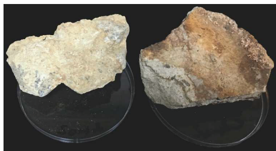
Fig. 1. Typical view of concrete samples from the walls of the shop for the production of titanium dioxide by the sulfate method
