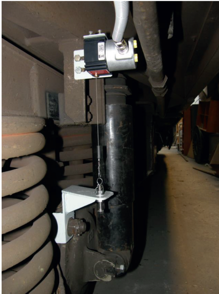
Figure 3. The wire position sensor measuring the vertical deviation of the wagon body from the wheel axis.
