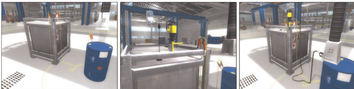
Figure 10. A pump is installed, grounding cables are attached, and a pipe leads to the barrel.
