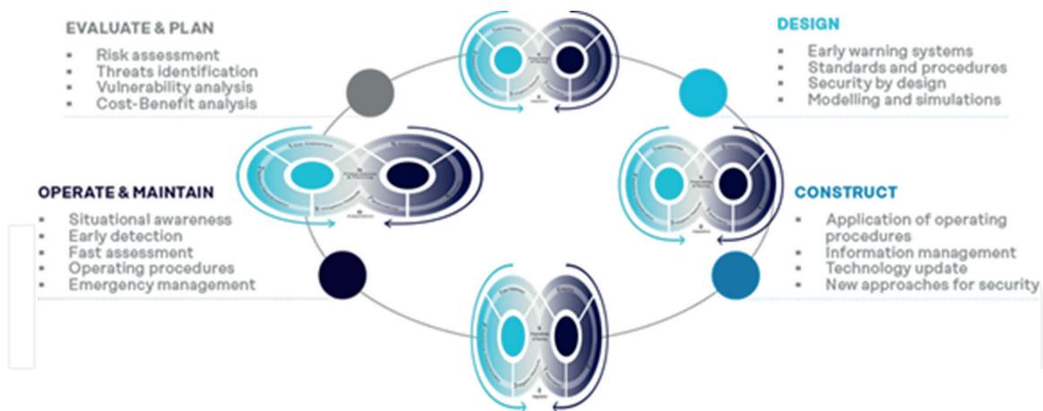
Figure 7. Brief representation of the resilience management process across the life cycle of an infrastructure followed from RINA, where the proposed methodology is contributing to the design and evaluate and plan phase (source: RINA).
