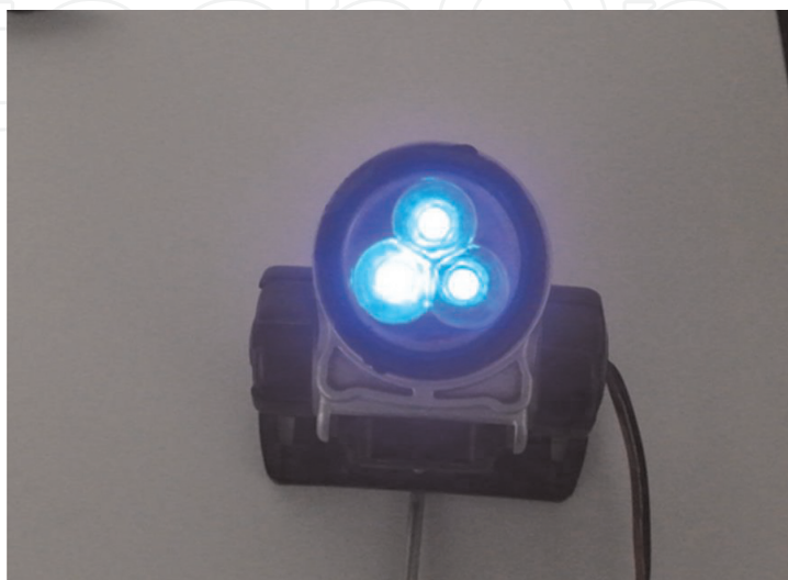
Figure 4. LED lights are energized with a melanin-based battery.
