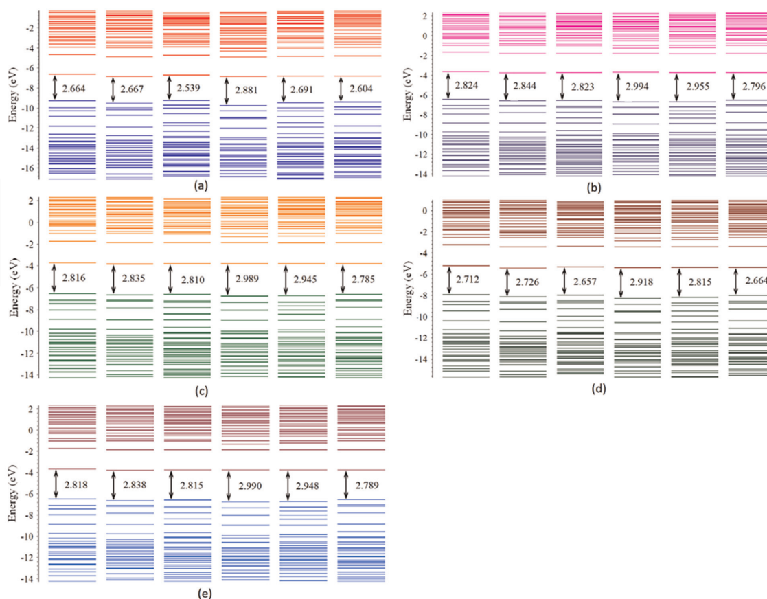
Figure 2. Molecular orbitals for selected anthocyanidins cyanidin [22], delphinidin, malvidin [22], pelargonidin, peonidin [22], and petunidin corresponding to (a) gas phase, (b) water solvent, (c) ethanol solvent, (d) n-hexane solvent and (e) methanol solvent. H-L gap energy units are in eV.
