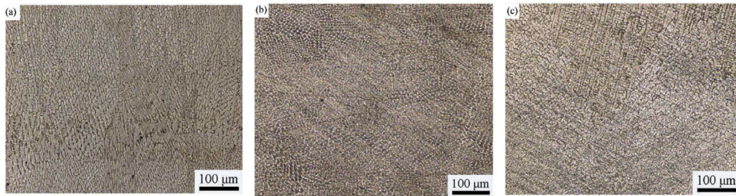
Fig. 15. Microstructure of ASHM in (a) bottom zone, (b) middle zone, and (c) top zone of the product [129].
