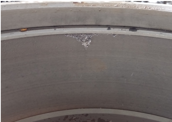
Figure 4: Photograph of spall formation discovered on the IB raceway of Test Cup A after 51,420 miles of operation – 2 nd Teardown
