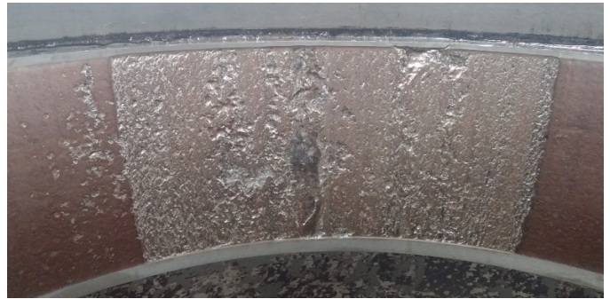
Figure 13: Photograph of the extensive spall degradation of the existing spall found on Test Cup C (Bearing 3) after running an additional 27,802 miles of operation – 10 th Teardown
