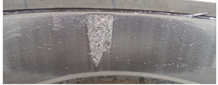
Figure 10: Photograph of further degradation of the existing spall found on IB raceway of Test Cup B of Bearing 3 following an additional 4,769 miles of operation – 7 th Teardown
