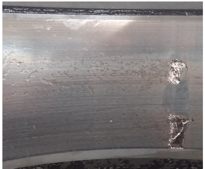
Figure 11: Photograph of the spall that developed on the IB raceway of Test Cup C of Bearing 2 after running a total of 214,452 miles – 8 th Teardown
