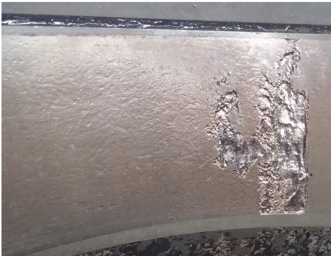
Figure 12: Photograph of the deterioration of the existing spall located on the IB raceway of Test Cup C after an additional 7,805 miles of operation – 9 th Teardown
