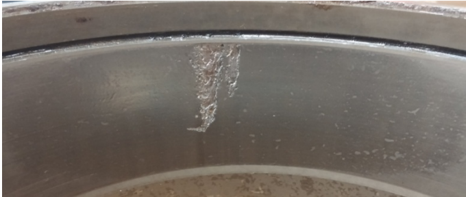
Figure 9: Photograph of the deterioration of the existing spall discovered on Test Cup B of Bearing 3 after running an additional 10,757 miles – 6 th Teardown
