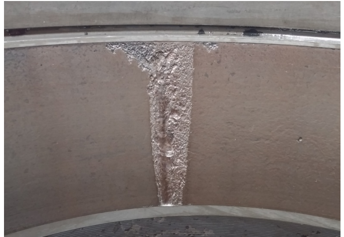
Figure 5: Photograph of degradation of the existing spall found on Test Cup A after running an additional 12,258 miles – 3 rd Teardown
