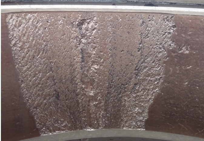
Figure 6: Photograph of further deterioration of Spall 1 on Test Cup A after operating an additional 13,828 miles — 4 th Teardown
