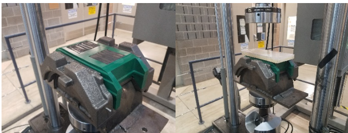
Figure 4: Prototype Polymer adapter steering pad on simulated bearing in material testing system
