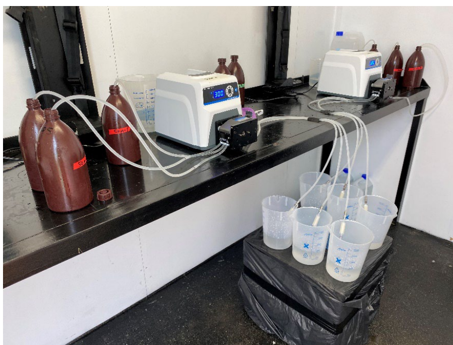
Figure 4. Simultaneous filtration of collected water samples inside the on-deck container using peristaltic pumps powered from electricity to the container. Triplicate 1L-water samples (brown bottles) from each sampling depth (50 m on the left, 10 m on the right) were filtered through 0.45 \mu\text{m} Sterivex filters using four-channel pump heads set to 300 rpm (flow rate approx. 100 mL min -1 ). Filter outflow was collected in 2L-beakers, and outflow volume was measured and recorded.
