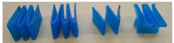
Figure 5: AM weirs (from left to right: empty catenary, ramped catenary, labyrinth, piano key).
