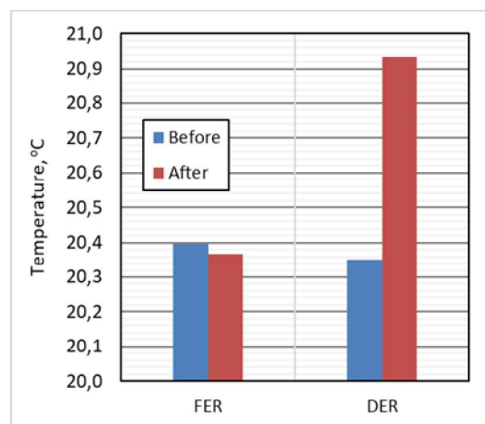
Fig. 4 – Temperature (coldest spot) before and after retrofits.
