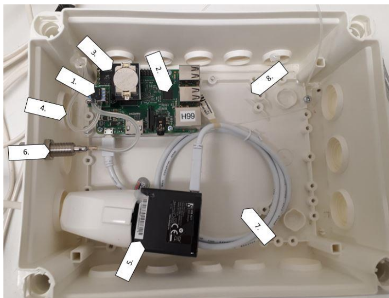
Figure 1. The air pressure difference measurement unit inside an installation box. 1. Differential pressure transmitter (Honeywell TruStability). 2. Raspberry Pi 2 model B. 3. Clock timer. 4. Flexible tube for differential pressure transmitter (indoor air conditions). 5. Power adapter for Raspberry Pi. 6. A coupler for different diameter tubes (outdoor air conditions). 7. Protective casing for the device. 8. Connection board (transparent plastic) to fix the equipment to the casing.
