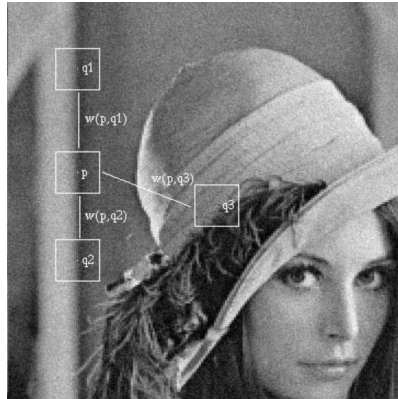
Figure 2.3. Scheme of NL-means strategy. Similar pixel neighborhoods give a large weight, w(p, q1) and w(p, q2) , while much different neighborhoods give a small weight w(p, q3) . [6]
