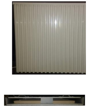
Figure 3: Sample B, radiator, clay chamotte core (a) electric radiator (b) core
