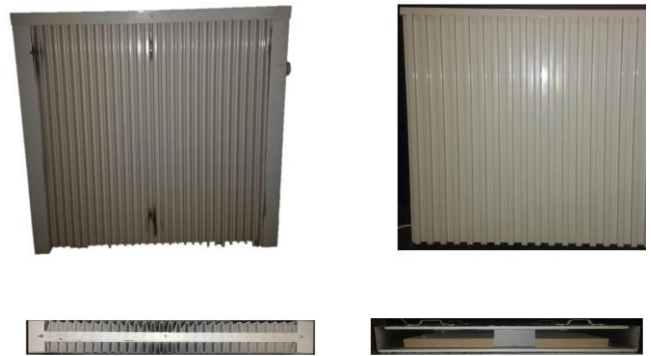
Figure 2: Sample A, radiator, fireclay core (a) electric radiator (b) core
