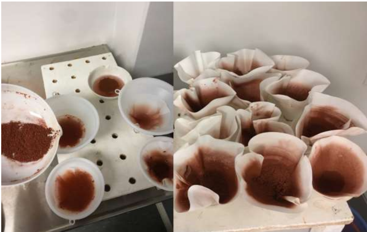
Figure 3.10 Left: stable aggregates poured over to funnels with VWR 415 filter paper. Right: air dry material, before weighing.
