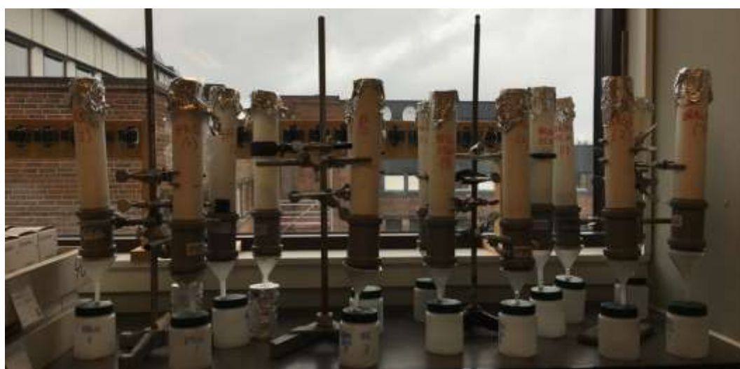
Figure 3. 7: Polypropylene (PP) columns used for aggregate stability studies. The funnels are fastened to the cap of the bottles. The aluminium cover is to reduce water evaporation.
