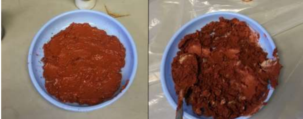
Figure 4. 10 Photographs taken of BR (left) and BR+10% gypsum (right) immediately after taking down the columns, three days after the last water addition.
