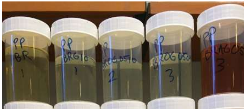
Figure 4. 3: Leachate colour after 400 mL water had percolated through the polypropylene (PP) columns (Most of the first 200 mL added was retained in the columns). From the left: 100% BR, 10% gypsum (G), 10%G, 5% Açai waste, 5%G, 5% Açai waste and 10%G, 5% food waste. The colour difference decreased as the leachate volume increased (increased L/S).
