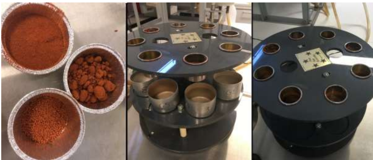
Figure 3.8 Left: the bottom aluminium container contains 1-2 mm aggregates. Middle and right: The Eijkelkamp's wet sieving apparatus, with 0.5mm sieves in the top tray and steel containers in the bottom tray.
