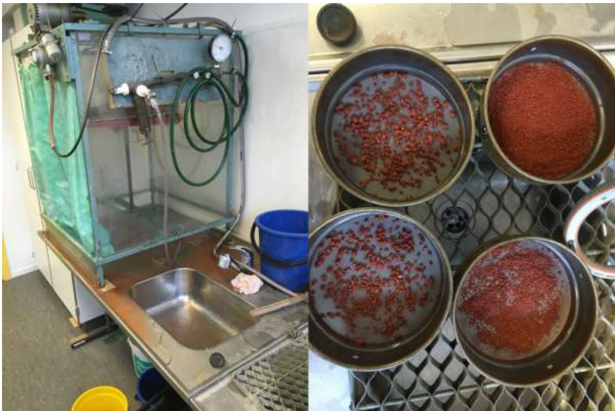
Figure 3. 9 Left: rainfall simulator cabinet with the rotating disk in the middle. Right: 2-6 mm and 0.5-2mm aggregates placed on 0.5 mm sieves, before they were placed in the cabinet of the rainfall simulator.
