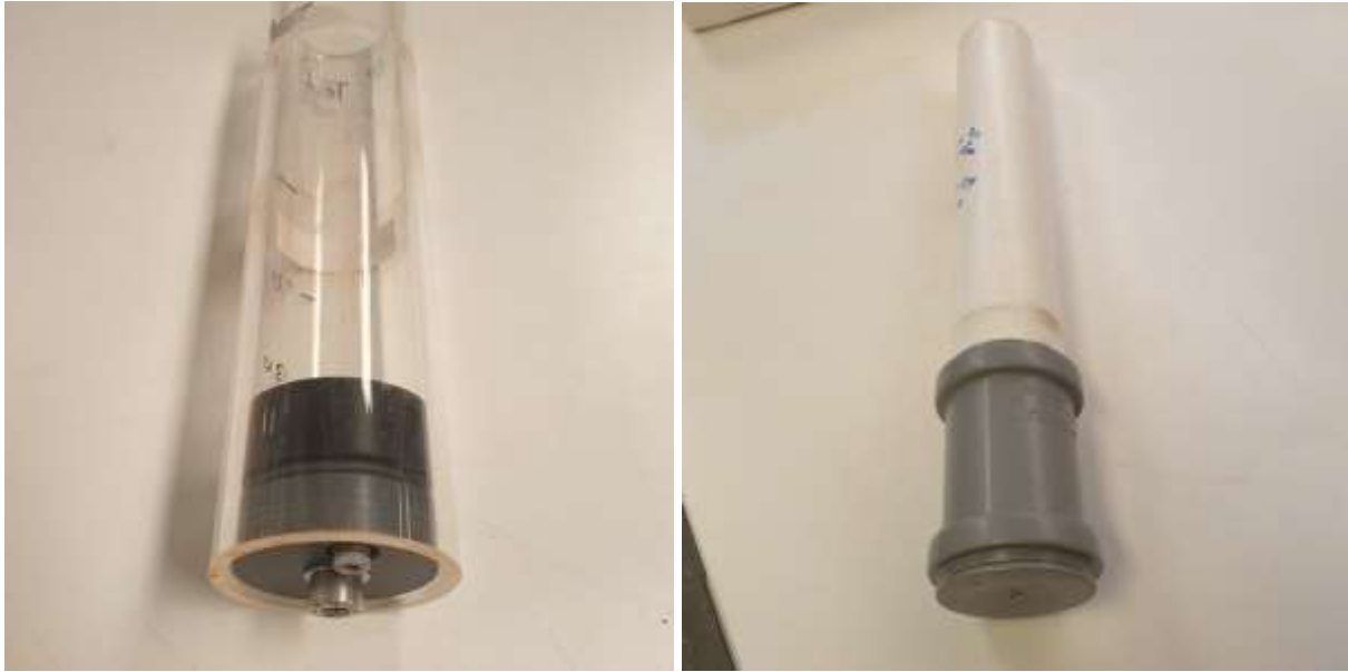
Figure 3. 6: Left: NGI columns, used for plant growth studies on leached BR material. Right: PP columns used for aggregate stability study prior to plant growth.
