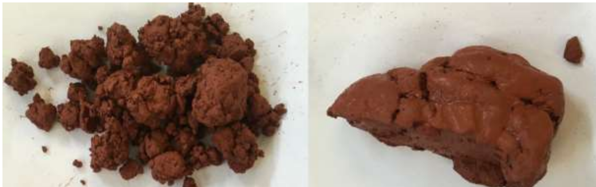
Figure 4. 9 Field moist bauxite residue from with 10% gypsum (left) and unamended BR (right). Samples taken prior to plant growth, approximately six months after application of gypsum (Y. Miura, 2022a).
