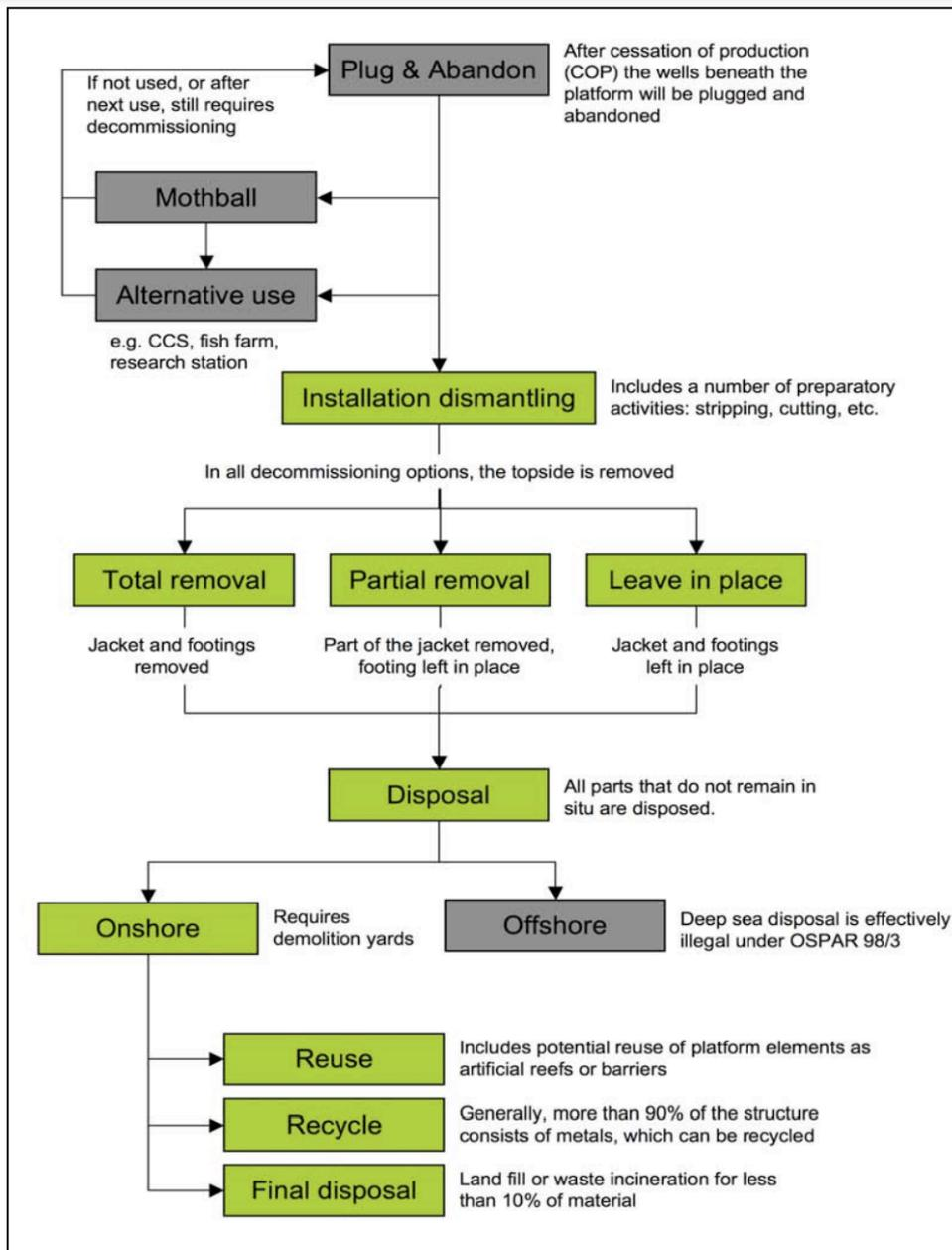
Figure 3.2: Overview of the decommissioning process with all three different options
