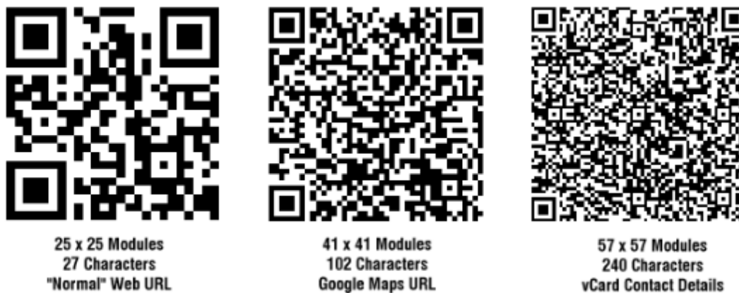
Figure 3.2: Trade-off between QR Code Size and Scanning Distance, Source: [33]
