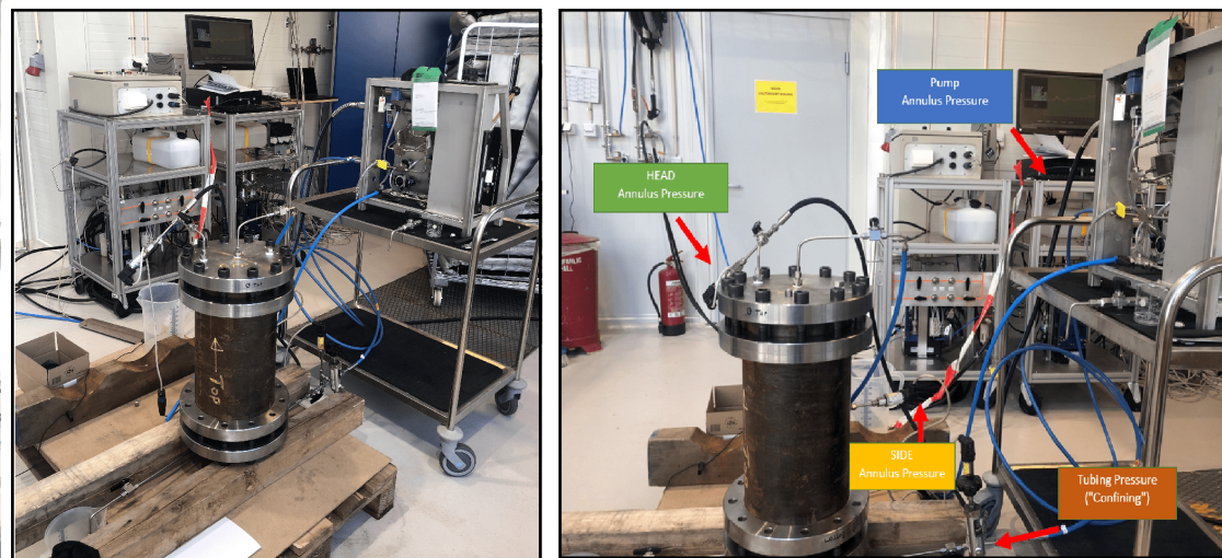
Figure 3.5: Picture of instrumentation and rig up for testing for the uniform debond cell
