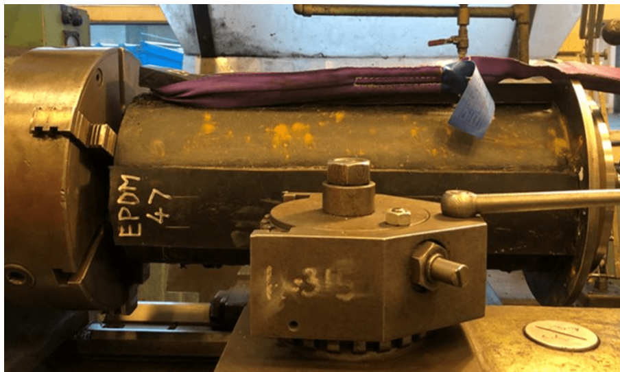
Figure 5.6: Crude test to evaluate the adhesive bond between the rubber materials and casing surface.
