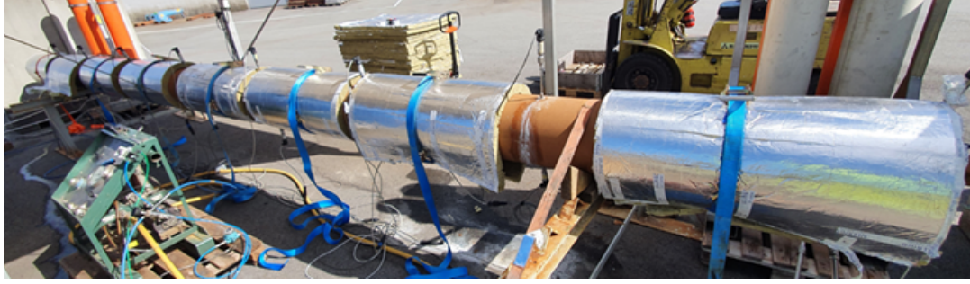
Figure 3.31: Typical instrumentation during leak testing on Transition Joint.
