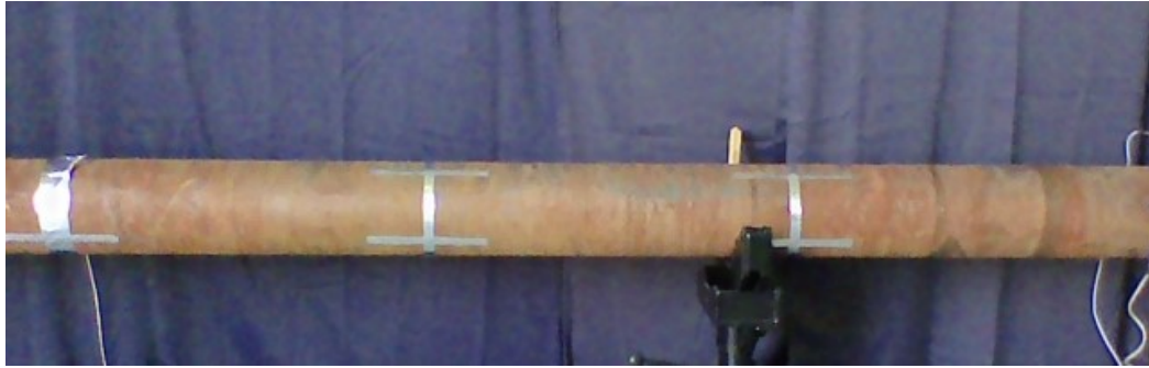
a) Test section C6 with metallic tape for position identification.
