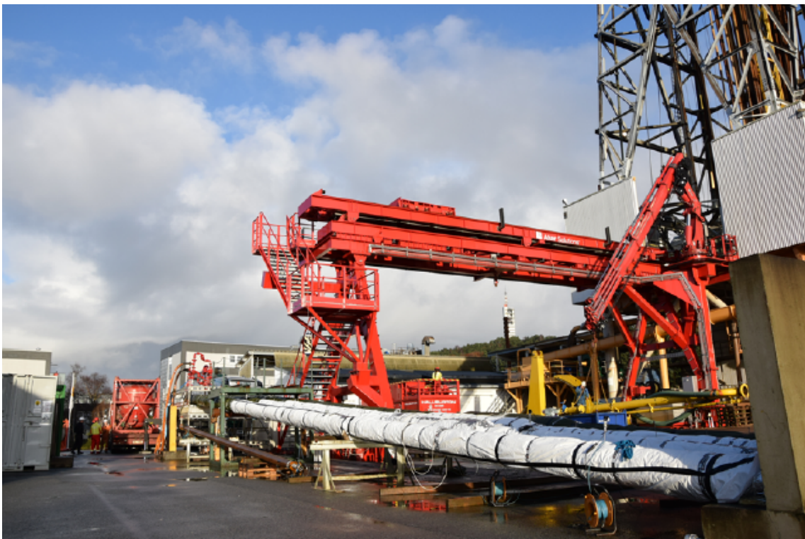
Figure 3.9: View of the four test assemblies draped in insulation and plastic covers.
