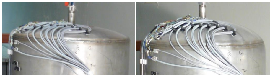
Fig. 9. Changes in the shape of the tank bottom at an increase of pressure up to 30 bar
