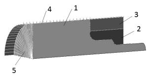
Fig. 2. Exemplary geometrical model of the analyzed extrusion process: 1 – formed material, 2 – die insert, 3 – prestressing ring, 4 – container surface, 5 – punch surface
