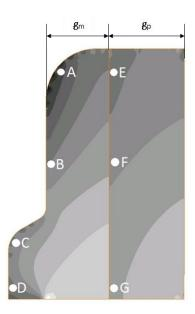
Fig. 3. Locations of measurement points of circumferential stresses
