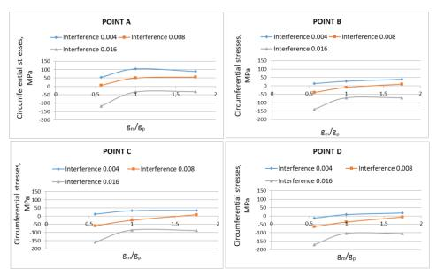
Fig. 4. The impact of the  $g_m/g_p$  quotient on the value of maximum circumferential stresses in individual areas of the die insert depending on the used assembly interference
