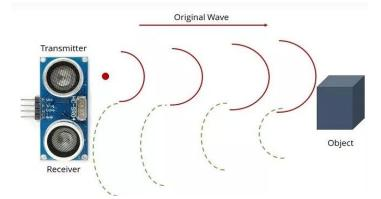
Fig. 5. Ultrasonic range detection
