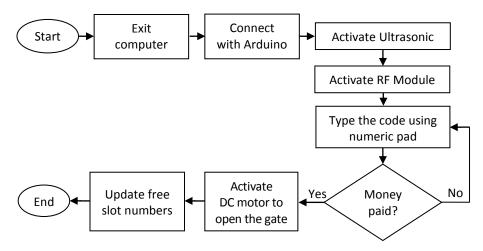
Fig. 9. Flowchart for the exit gate
