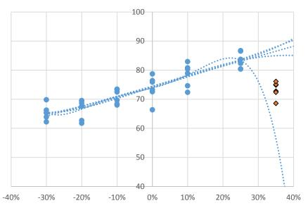
Fig. 2. Compressive strength of bone cement with a +35 % excess of the liquid component: comparison of mathematical models and experimental data
