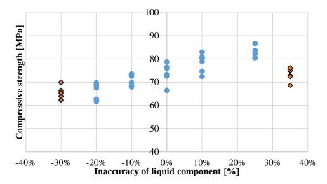
$\label{eq:Fig.1.} \textbf{Result from experimental research on compressive strength} \\$
