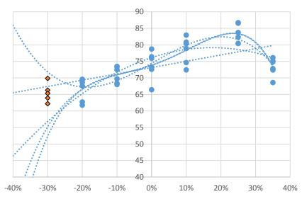
Fig. 3. Compressive strength of bone cement with a -35 % deficiency of the liquid component: comparison of mathematical models and experimental data
