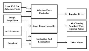
Fig. 6. The proposed system block diagram
