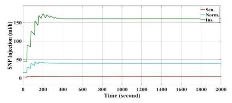
Fig. 9. SNP Injection according to the MRAC Optimized with GWO
