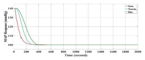
Fig. 7. The response of MAP according to the MRAC optimized with GWO
