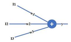
Fig. 2. The ADALINE Network Architecture
