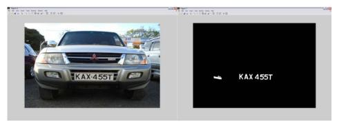
Fig. 1. Input image and the resulting extracted plate characters
