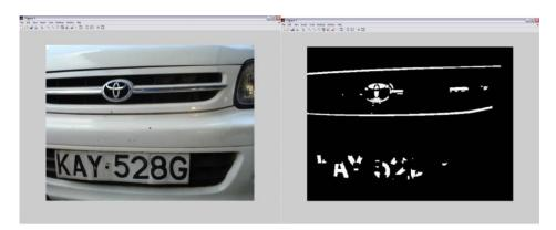
Fig. 9. Input image is too close to the camera
