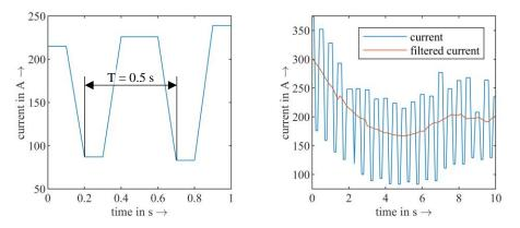
Fig. 5. Fluctuations in the current and raw and filtered current signal
