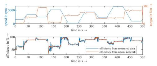
Fig. 10. Speed and torque corresponding to the efficiency from the measured data and the ANN
