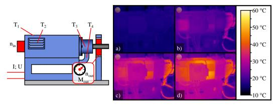
Fig. 3. Schematic illustration of the measurement locations and IR-illustration of the heating after: a) 0 min, b) 50 min, c) 100 min and d) 150 min
