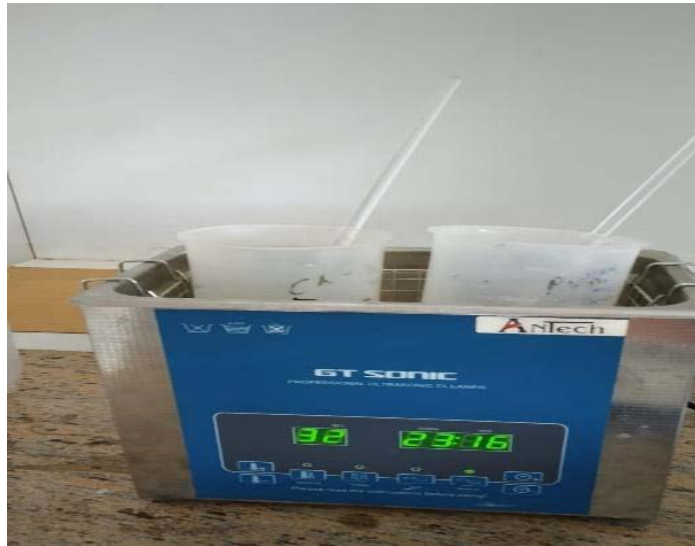
Fig. 1: Formulation placed on ultra-sonication to remove air bubble
