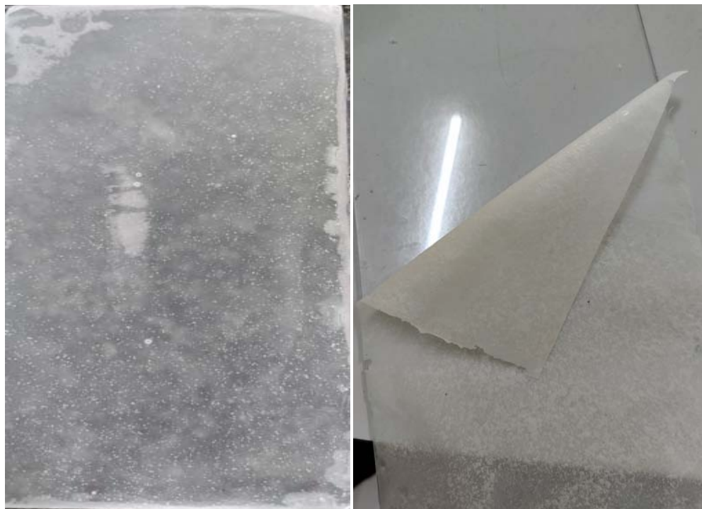
Fig. 2: After the drying film removed from the film former
