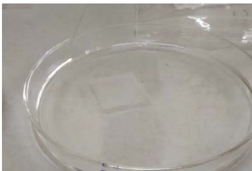
Fig. 4: Film placed in petri plate for disintegration
