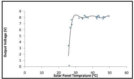
Solar panel efficiency was observed to increase with rise in temperature (figure 3). A maximum efficiency of about 87.0% was obtained at a solar panel temperature of 43.8°C. Further increase
