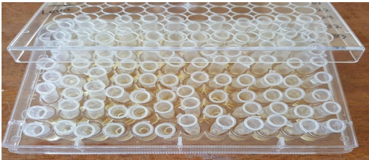
Figure 1. Bacterial suspension with autoclaved pegs to act as surface for biofilm growth
