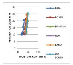
Figure 4: Atterberg limit of the soil samples
