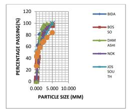
Figure 3: Sieve Analysis of the soil samples
