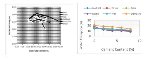
Figure 5: Compaction test of the soil samples
