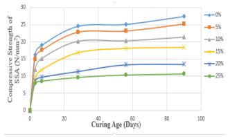
Fig. 6: Relationship between Compressive Strength and Curing Age
