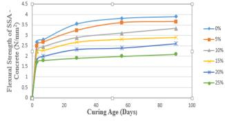
Fig. 7: Relationship between Flexural Strength and Curing Age
