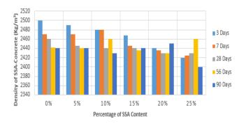
Fig. 8: Relationship between Density of SSA-Concrete and Percentage of SSA Content
