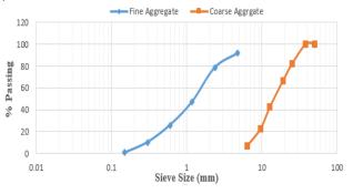
Fig. 1: Particle Size Distribution of Fine and Coarse Aggregates
