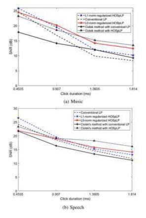
Figure 4: SNR of restored audio by using detection and restoration without any a priori knowledge on location and duration of click degradation.
