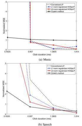
Figure 2: Performance of click duration estimation at 44.1 kHz sampling frequency.
