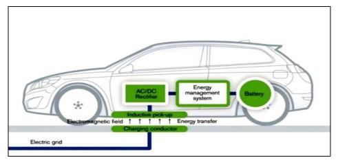
(Source: https://www.motorbeam.com/wp-content/uploads/Volvo-Electric-Vehicle-Cordless<u>https://www.motorbeam.com/wp-content/uploads/Volvo-Electric-Vehicle-Cordless-Charging-Technology.jpg</u>Charging-Technology.jpg) **Figure 2.** The representation of Induction Charging.
