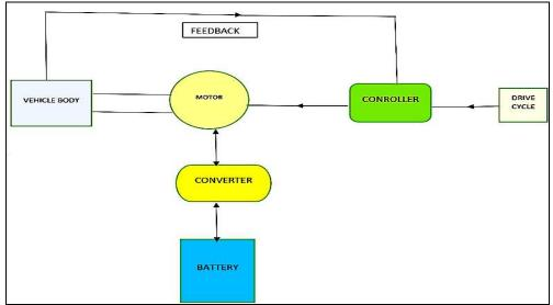
Figure 1. The general block diagram of an Electric Vehicle.
