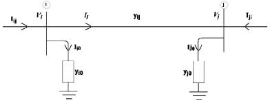
Figure. 1. Transmission line model for calculating the power loss.
