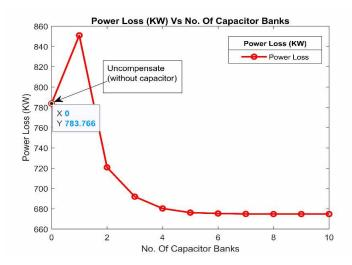
Figure 4. Power Loss (KW) Vs No. Of Capacitor Banks.
