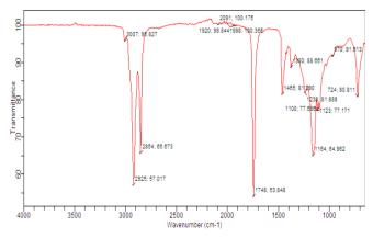
Figure 4. FT-IR Spectra of Transesterified Neem Oil
