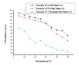
Figure 2: graph of viscosity against Temperature
