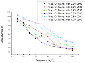
Figure 3: Graph of Viscosity of Nano fluid against Temperature
