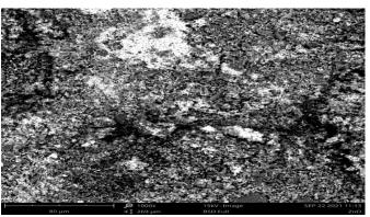
Figure 1: SEM of Zinc oxide at the Magnification1000X
