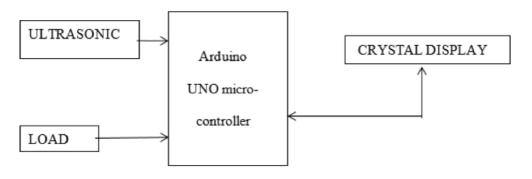
Figure 6: BMI Measuring Device Block diagram.
