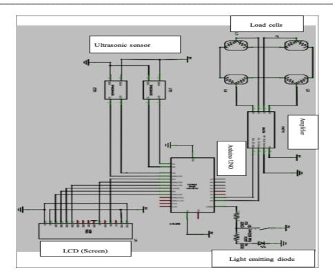
Figure 1: BMI Measuring Device Circuit diagram.
