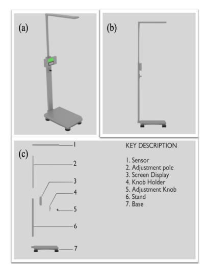
Figure 3: (a) Pictorial representation of the proposed BMI device using BLENDER software. (b) Side view of the BMI device using BLENDER software. (c) Exploded view of the BMI device using BLENDER software.
