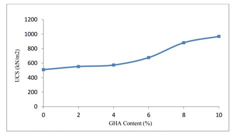
Fig. 3.4 - UCS values measured as a function of GSA values added
