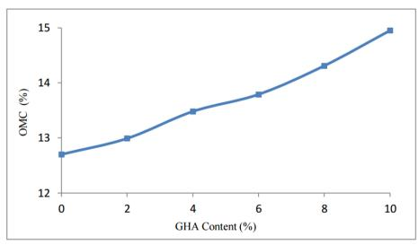
Fig. 3.2 - OMC values measured as a function of GSA values added
