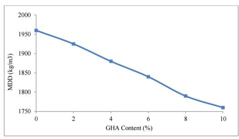
Fig. 3.1 - MDD values measured as a function of GSA values added
