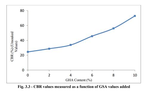
Thus, according to figure 3.3, the CBR value rises from 24.42 percent at 0% GSA to 72.88 percent at 10% GSA as soil weight increases. The progressive appearance of cementitious compounds in the soil due to the interaction between GSA and a particular calcium hydroxide in the soil may be the cause of this rise[9]. The findings demonstrated that GSA stabilization significantly boosted the samples' strength in terms of their samples.
