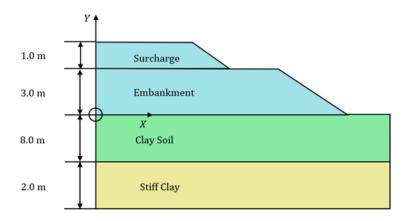
Fig.1 - Geometry of the proposed model
