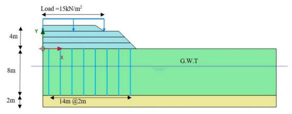
Fig. 2 - Conventional model with surcharge
