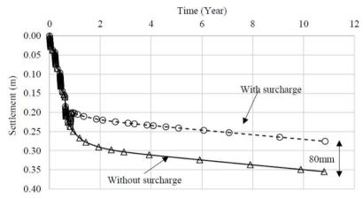
Fig. 5 - Settlement prediction of full stage construction of embankment with and without surcharge
