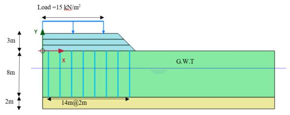
Fig. 3 - Conventional model without surcharge
