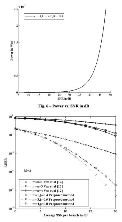
Fig. 7 – Comparison of ABER vs average SNR between the proposed system over *K*<sub>G</sub> fading channel and that given in Van et.al [12] for Nakagami fading channel
