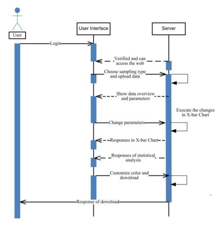
Fig. 3 - Interaction design in UML for user interface (UI)
