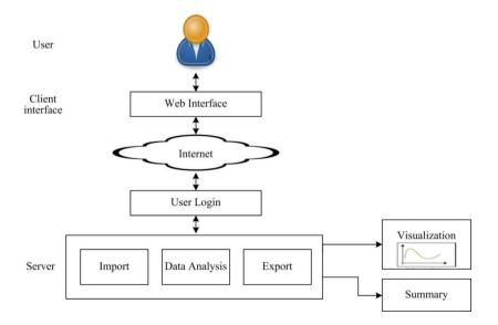
Fig. 4 - Web-based software system architecture
