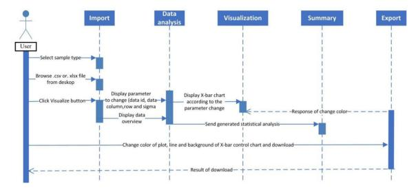
Fig. 5 - Interaction design in UML for SPC analysis
