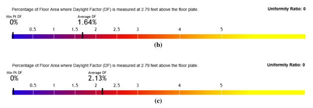
Fig. 10 - Average Daylighting Factor (ADF) of the units (a) twodio unit; (b) three-bed unit; (c) four-bed unit
