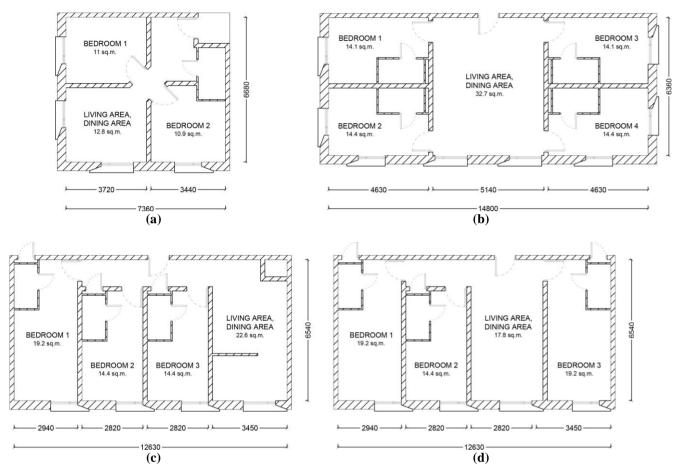
Fig. 6 - Floor plan of the co-living units (source: Manchester City Council, 2018) (a) twodio type; (b) 4-bed type; (c) 3-bed type 1; (d) 3-bed type 2
