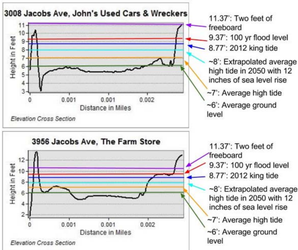
Figure 10. Cross sections of vulnerable (John’s Used Cars & Wreckers) and structurally sound (The Farm Store) portions of levee with associated thresholds of significance. Satellite imagery and a 1-meter resolution Digital Elevation Model (DEM) of the landscape shows the average ground height in the Jacobs Avenue basin to be approximately 6 feet. High tide stage heights at the Eureka Slough Bridge record at 4.75-8.5 feet, varying throughout the year, placing the high tide at approximately 7 feet (ProTides, 2011) (representation created using NAIP imagery and NOAA LiDar data).
