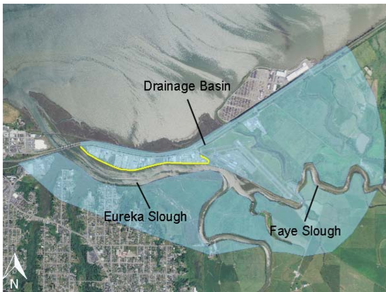
Figure 11. Eureka Slough hydrologic unit, an area of interconnected waterways experiencing shared impacts of tidal fluctuations. A levee failure in Faye Slough could bring about flooding on Jacobs Avenue regardless of levee improvement efforts due to the unarmored eastern edge and the tract's basin-like topography (data derived from NAIP imagery; NOAA LiDar; Laird, 2013; and Laird, personal communication, 2013).
