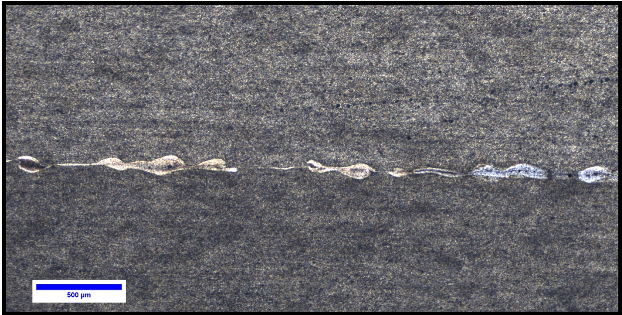
Figure 5-6: Optical image of the 0.5° bond. Defects (cracks & voids) are visible. Frequent and sometimes relatively thicker melting, as much as roughly 100 μm, appear along the bond. However, some regions of thin, abrupt bonding appear.
