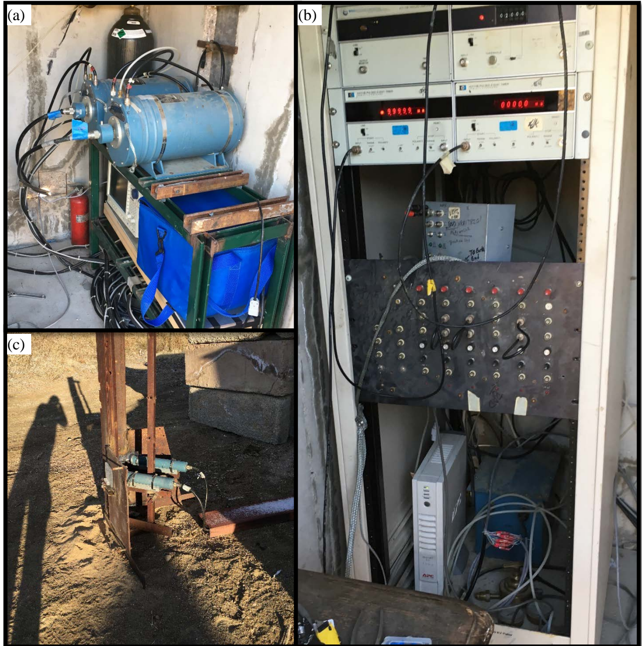
Figure 3-14: Flash X-Ray system used in testing. a) Charging components. b) Discharge delay system. c) Protective cover guarding X-Ray head connecting to larger leads in a).
