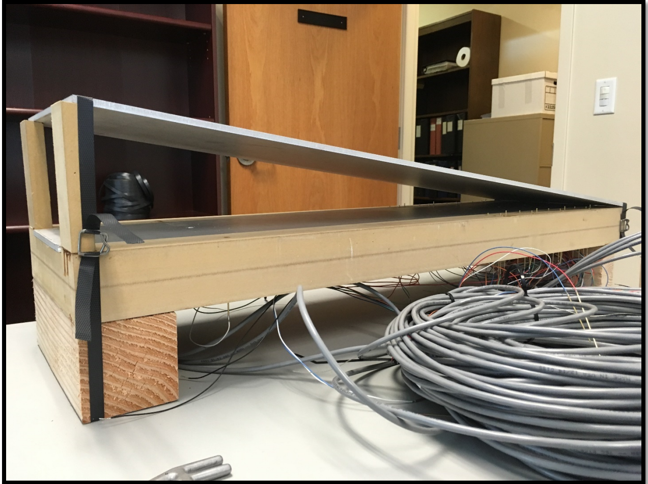
Figure 3-1: Example test specimen (8 degree without explosive and explosive instrumentation.)
