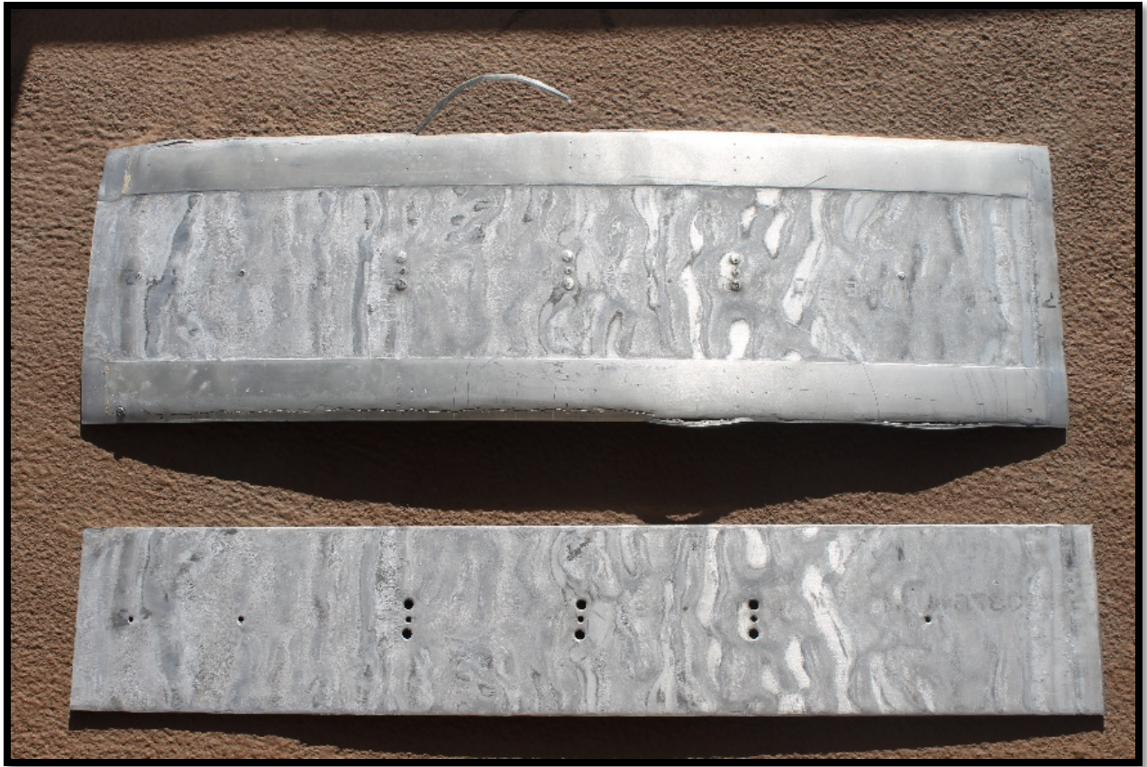
Figure 3-25: 0.5°, non-annealed, make-up test that failed to weld
