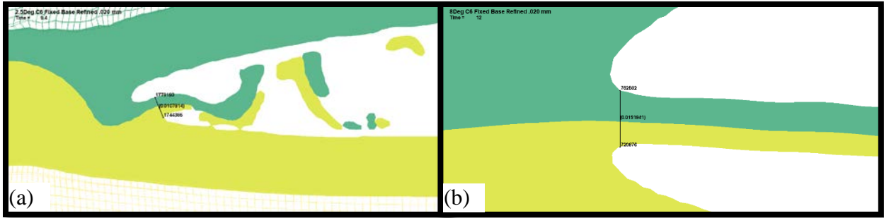
Figure 6-5: Jet thickness from modeling. Distances labeled inside of the parentheses are in cm. (a) 2.5° case. (b) 8° case.
