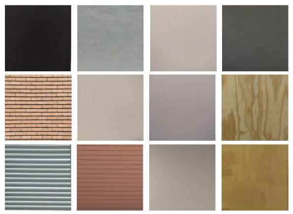
Figure 6 – Test Targets (left to right, top to bottom): Black Foam, Gray Stucco Wall\*, Gray Tabletop, Gray Painted Wall\*, Red Brick\*, Brown Paper, White Poster Board, Plywood, Silver Door\*, Brown Door\*, White Painted Wall, Corkboard.
