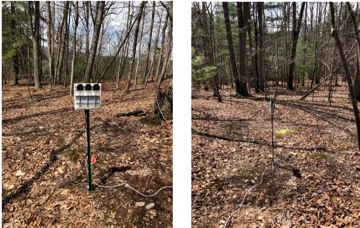
Figure 167. One remote firing device containing three remote firing mechanisms mounted on a steel u-post located in the wooded forest at the field localization site (Left: Front view of remote firing device, Right: Profile (side) view as seen from direction of the participant), which reduced the visual signature.
