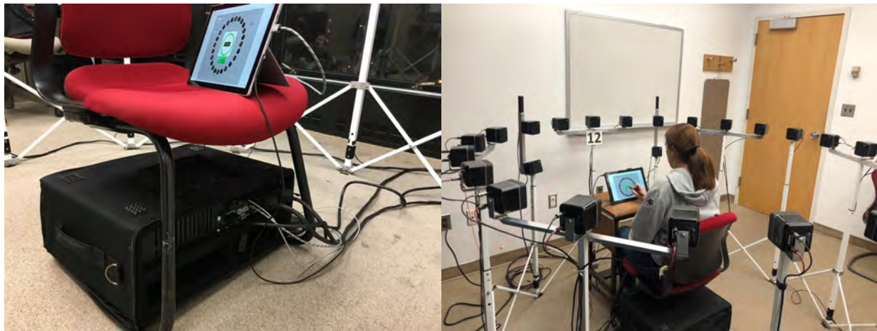
Figure 52. Microsoft® Surface Pro tablet user interface and audio case (left) and a trainee operating the PALAT system via tablet user interface (right).
