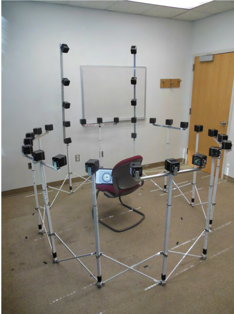
Figure 34. Fully expanded PALAT system frame with 32 loudspeakers.
