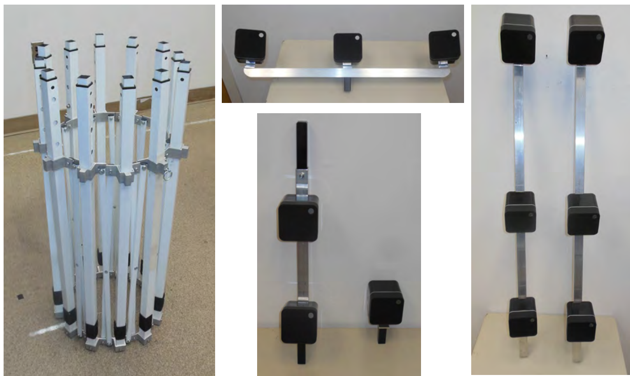
Figure 35. Collapsed PALAT system frame (left), three loudspeaker mount (top center), two loudspeaker elevation mount and single loudspeaker mount (bottom center), and elevation loudspeaker mount (right).
