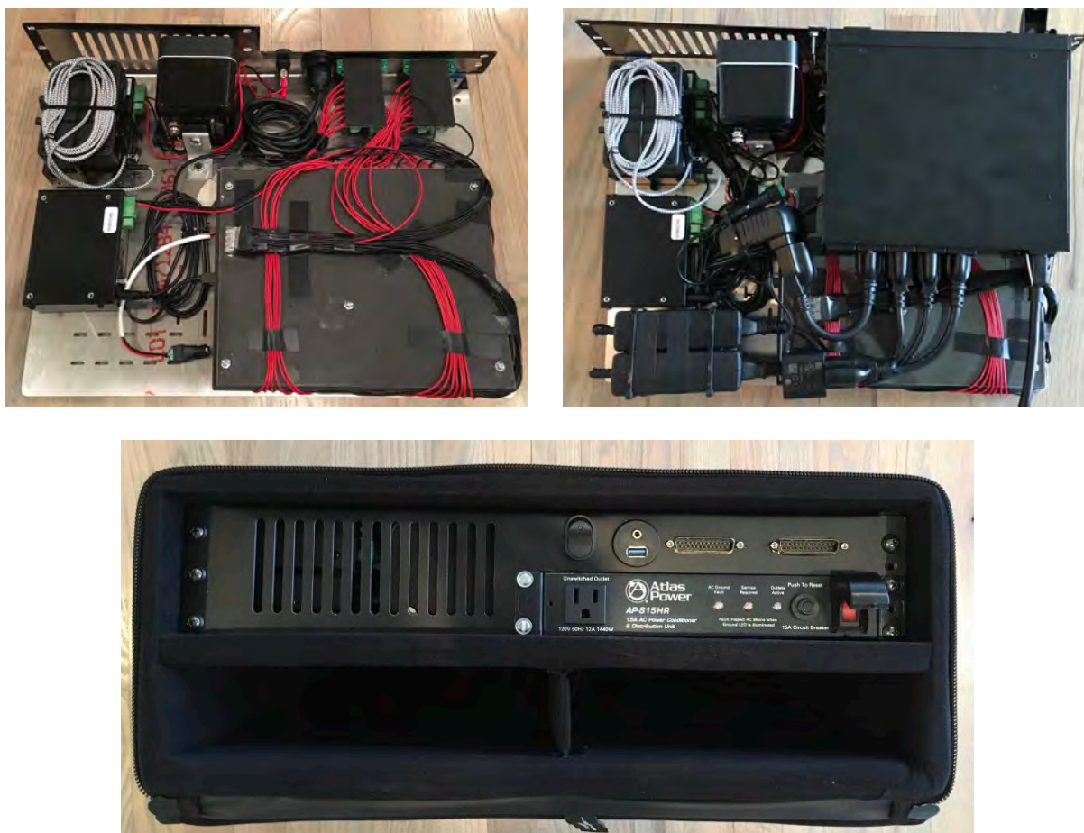
Figure 49. Audio components mounted to a custom audio rack (top left and right) and mounted in audio equipment bag (bottom).
