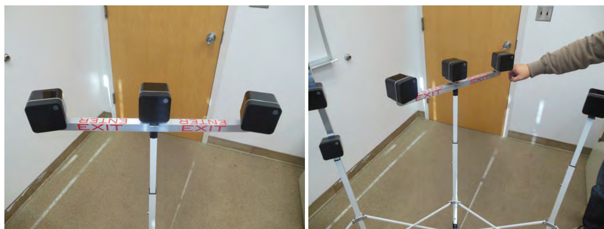
Figure 36. PALAT system entry/exit spring-loaded swivel gate loudspeaker mount.
