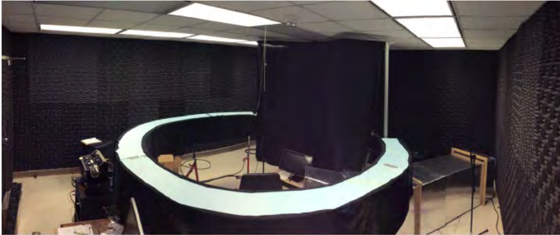
Figure 29. VT-ASL DRILCOM test apparatus located in the hemi-anechoic test room.
