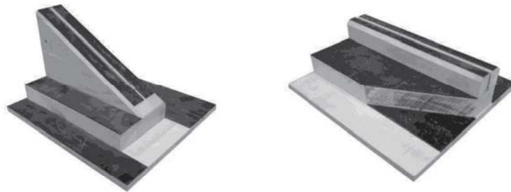
Figure 2: Blade holders, left: for closing positions, right: for closed flight and landing positions.
