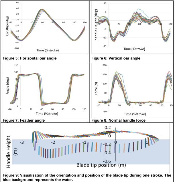
**DISCUSSION:** The RowIMU unit was easy and quick to set up on the course and was successful in measuring and storing the three oar angles and oar handle force. Importantly, the method used to calculate the oar angles in the RowIMU reports the true horizontal angle of the oar independently of the vertical and feather angle. Further, there is no need to mount custom gates on the boat pin in order to measure oar force as in other systems.
