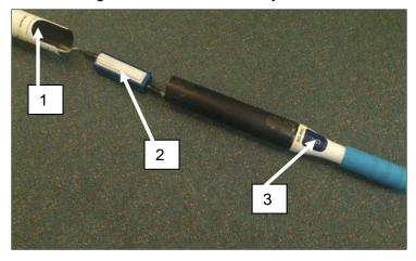
**Figure 1**. Dismantled Instrumented oar. Paddle with strain gauge force sensor (1). RowIMU module (2). On/Off switch, mode LED and charging port (3).
