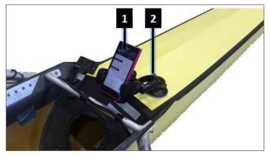
Figure 2. Smartphone (1) mounted on rowing shell (2).
