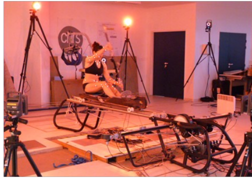
Figure 3: The Poitiers-B kayak ergometer equipped with the instrumented paddle shaft paddled by the elite female kayaker.
